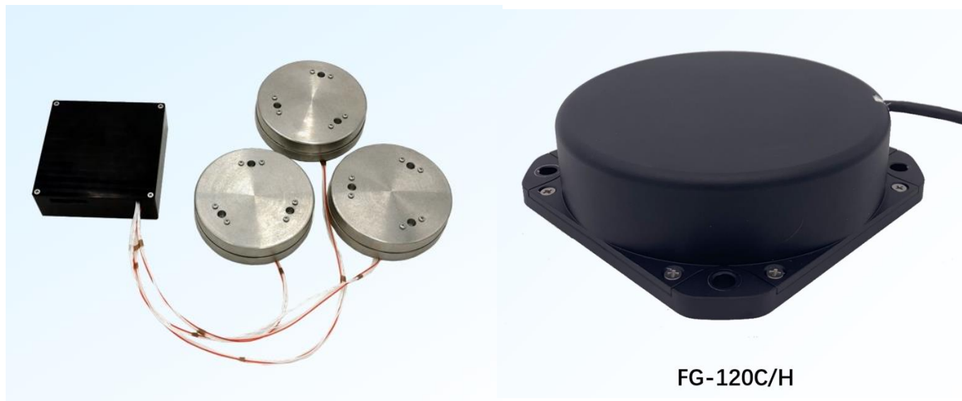
picture 1 FG-120C fiber optic gyroscope appearance and installation diagram
